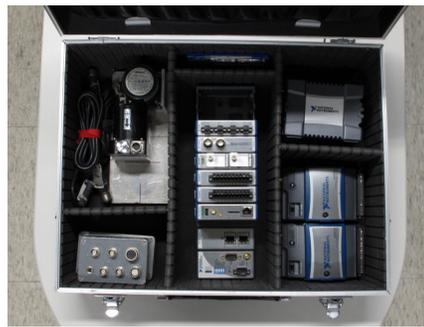
Fig. 9. The bridge health monitoring prototype
