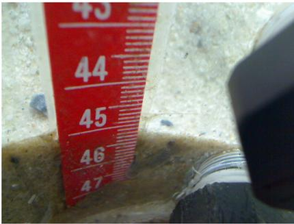
Fig. 8. The embedded depth monitored by camera
