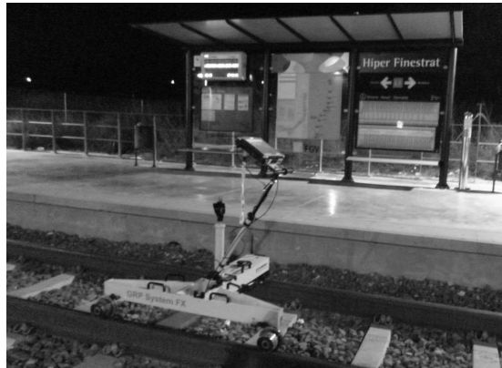
Fig. 3. Track surveying trolley at Hiper Finestrat station
