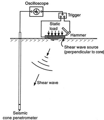
Fig. 2. Scheme of seismic cone penetration test [2]
