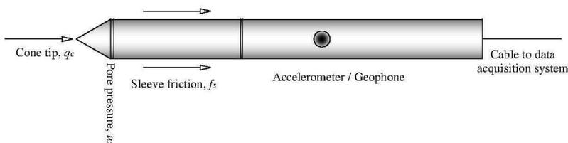
**Fig. 1.** Scheme of SCPT penetrometer
