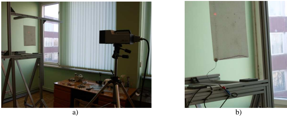
Fig. 4. Plate modal analysis experimental system: a) scanning laser system; b) hanged plate with connected piezoactuator
