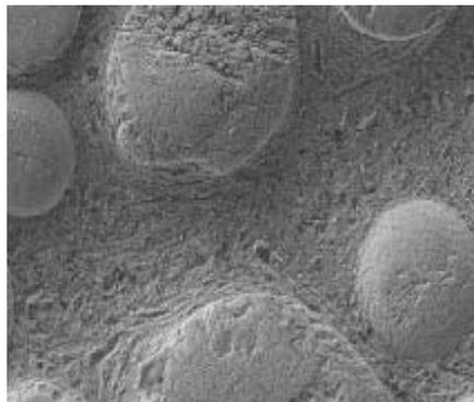
**Fig. 3.** Spheroidal carbides as components of standard padding materials [6]
