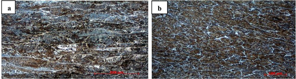
**Fig. 1.** The structure of the joint: a) after laser welding; b) after laser welding with the use of TiCN + Cu nanopowder [5]
