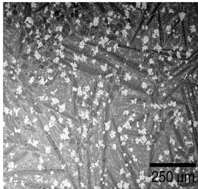
**Fig. 2.** Microstructure of EnDOtec TO \* 390 padding wire [6]
