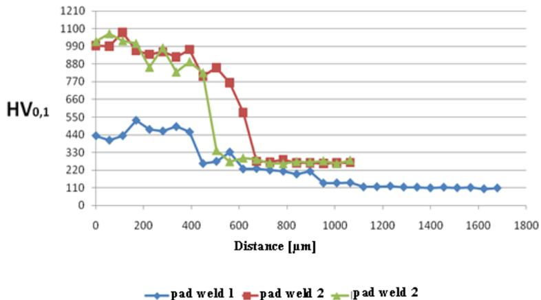
**Fig. 6.** Microhardness distribution in the cross-section of the padding weld created using the laser technique on 0H18N9 acid-resistant steel with the use of nanowire at various parameters of the process (from Table 3)
