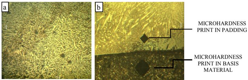
**Fig. 5.** Microstructure of the padding weld performed with the laser technique: a) zone of the padding weld material, b) penetration zone with the visible imprints of the microhardness tester at a load of 100G
