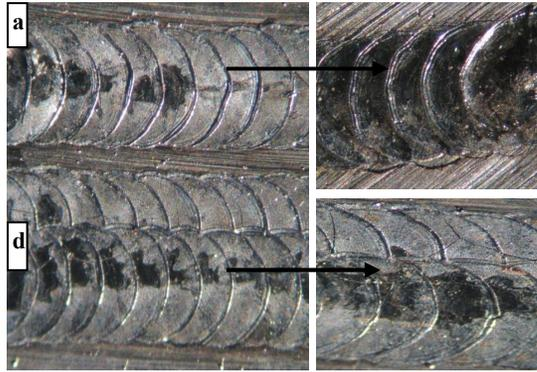
**Fig. 4.** Padding welding performed using laser technology with powder nanowire on 0H18N9 steel (variants “a”, “d” presented in Table 4)
