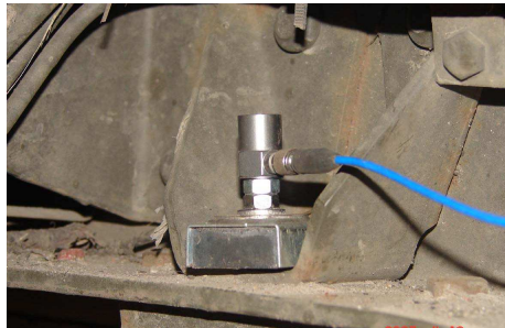
Fig. 3. Accelerometer attached with use of magnetic mat
