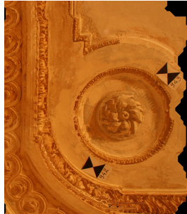
Fig 8. Orthophoto of the ceiling composed using object TIN data
