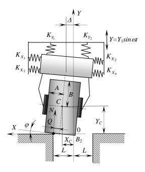
Fig. 2. Dynamic model of vibratory alignment
