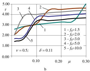
Fig. 3. Dependencies of parts alignment duration on: a – initial pressing force  $f_0$ ; b – friction coefficient  $\mu$
