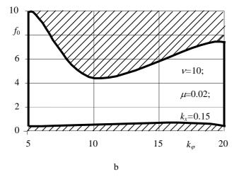
Fig. 4. Dependencies of parts alignment duration  $\tau$  on parameter  $k_{\varphi}$  (a); defined area of stable alignment of the parts (unhatched) depending on parameters  $k_{\varphi}$  and  $f_0$  (b)
