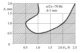
**Fig. 7.** Area of stable alignment of rectangular cross-section parts (unhatched) depending on excitation amplitude and initial pressing force
