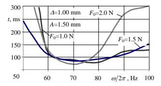
**Fig. 6.** Dependence of rectangular parts alignment duration t versus excitation frequency
