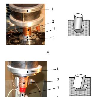
Fig. 5. Experimental setup for cylindrical (a) and rectangular cross-section (b) parts alignment
